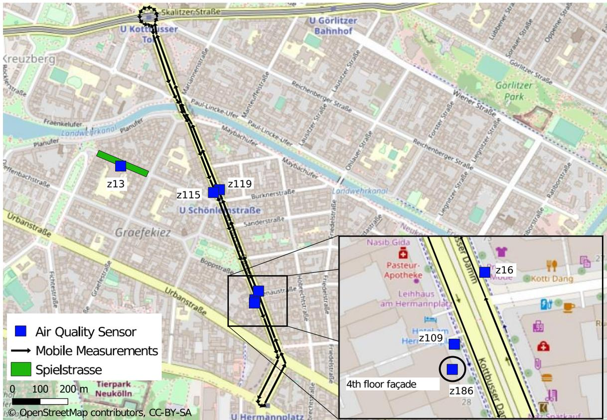
**Figure 3.** Air quality measurements on and around Kottbusser Damm. The stationary air quality sensors (blue squares) were mounted on lampposts or building façades. Sensor z13 was located on the 1<sup>st</sup> floor façade of the Lemgo primary school.
