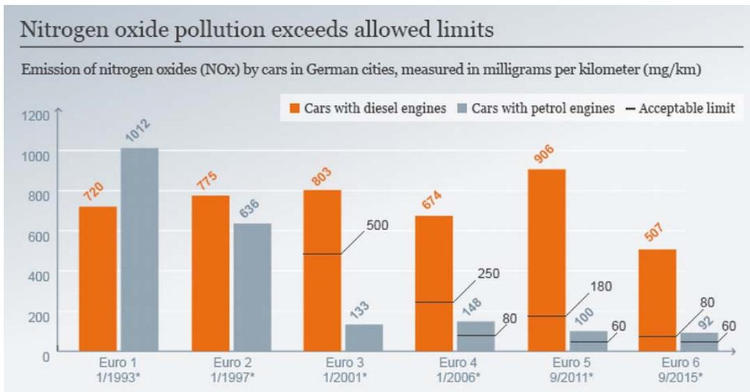
**Figure 2: A comparison of NO<sub>x</sub> emissions from petrol and diesel cars**
